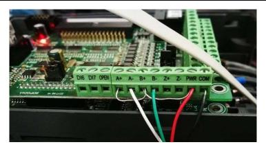
Step2, set encoder power voltage jumper and terminal DI6 < DI7 jumper as follows:
